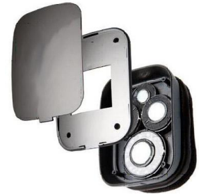
Figure 3.1: Multiple speakers placed around each ear.
